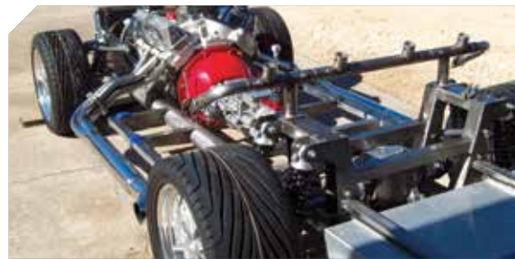
Cromgard C12 is used throughout the Shelby Cobra replica including the chassis.
